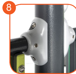
8 System of connectors and clamps made of strong aluminum alloy. Aluminum is secured by the process of electrophoresis and powder coating with polyester paint UV resistant and QUALICOAT attested.
